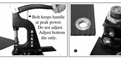
3) Place material between die and press handle all the way down
