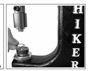
2) Place grommet on spring loaded pin of top die and washer on bottom die
