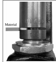
1) Adjust die to approximate thickness of material to be grommeted
